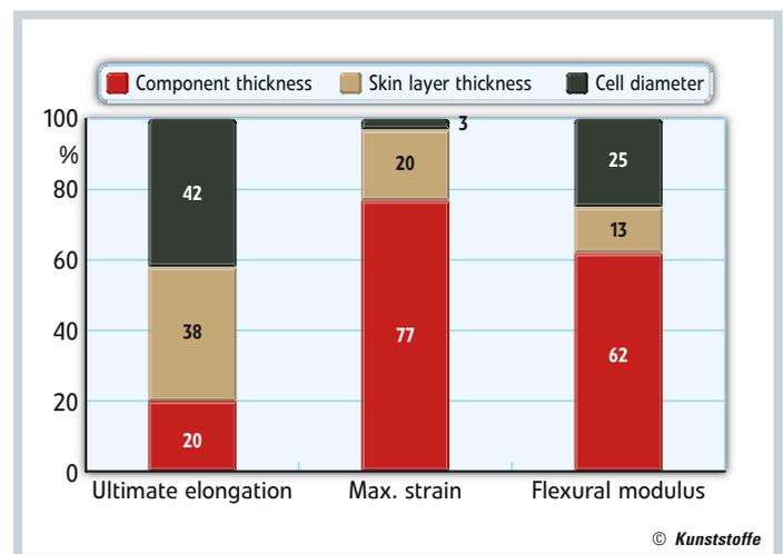
Fig. 3. Tensile stress for a component of polybutylene terephthalate (PBT): The graphic presentation shows that tensile properties are largely determined by the component thickness (strain and flexural modulus). Ultimate elongation mainly depends on the thickness of the skin layer and on the cell diameter. A coarse cell structure and low skin layer thickness reduce ultimate elongation (source [4]: IKV Aachen)
