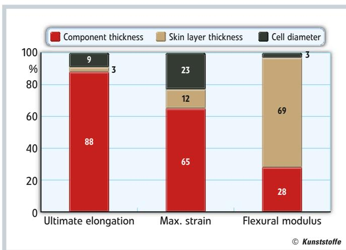
Fig. 2. Bending stress acting upon a component of polybutylene terephthalate (PBT): The graphic chart shows the skin layer thickness determining the flexural modulus, while component thickness is the crucial influencing factor to strain and ultimate elongation (source [4]: IKV Aachen)
