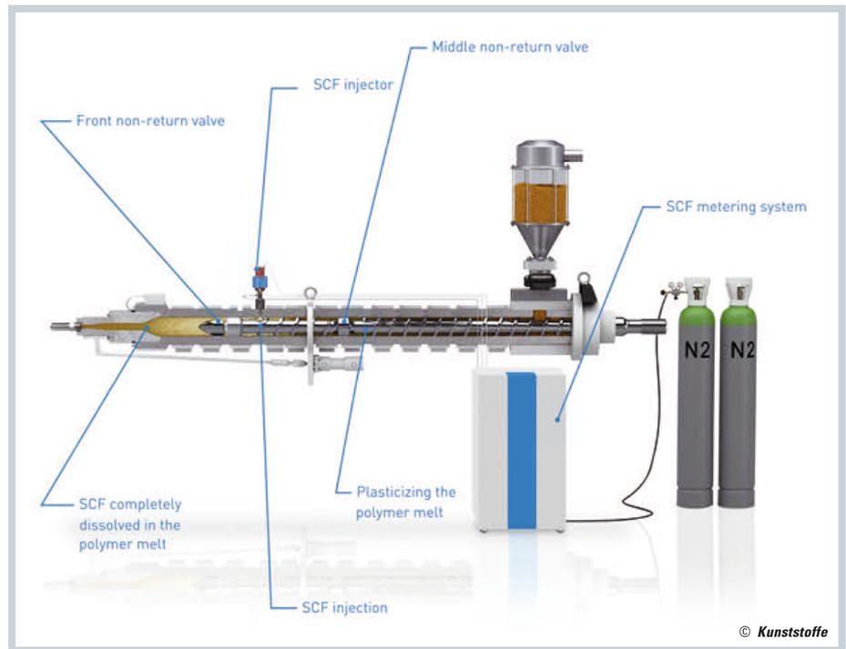
Fig. 1. Schematic presentation of a MuCell plant: The inert gas is dosed into the front third of the plasticizing unit, as a supercritical fluid (SCF) (figure: KraussMaffei)
