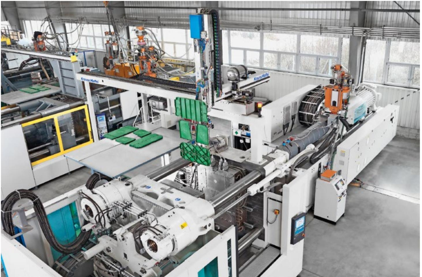
The internal parts of the three-phase composter Aeroplus 6000 are produced on the MX 1000-24500 with 150 mm Mucell screw and the LRX350 handling. Photo: Krauss Maffei
