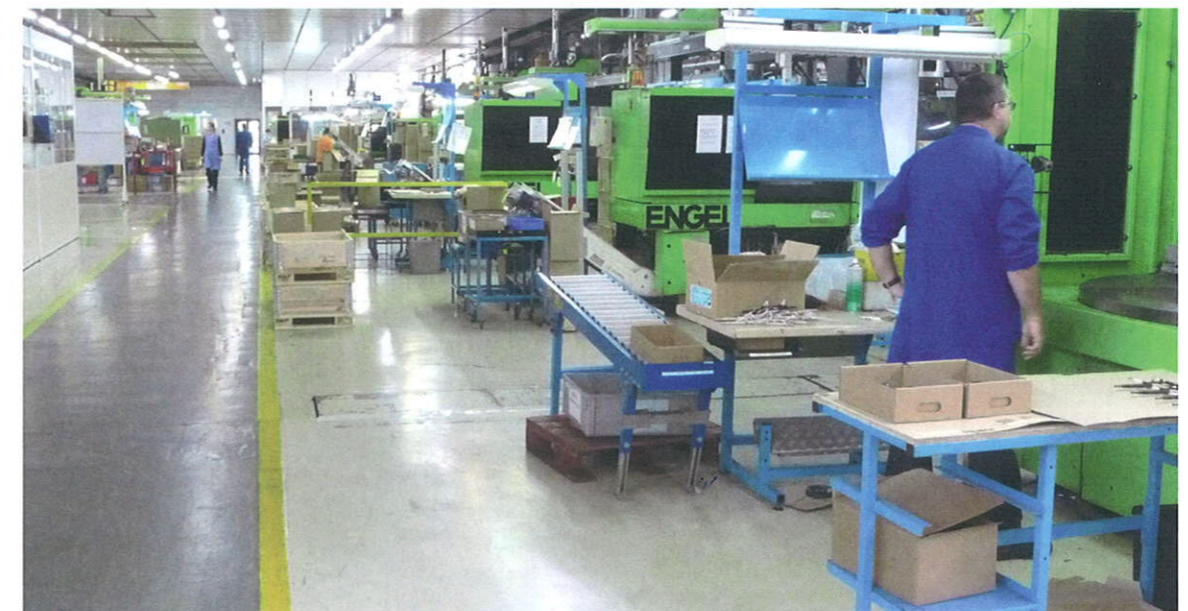
The machine park in Langeais contains 55 mostly tie-bar-less injection moulding machines.
