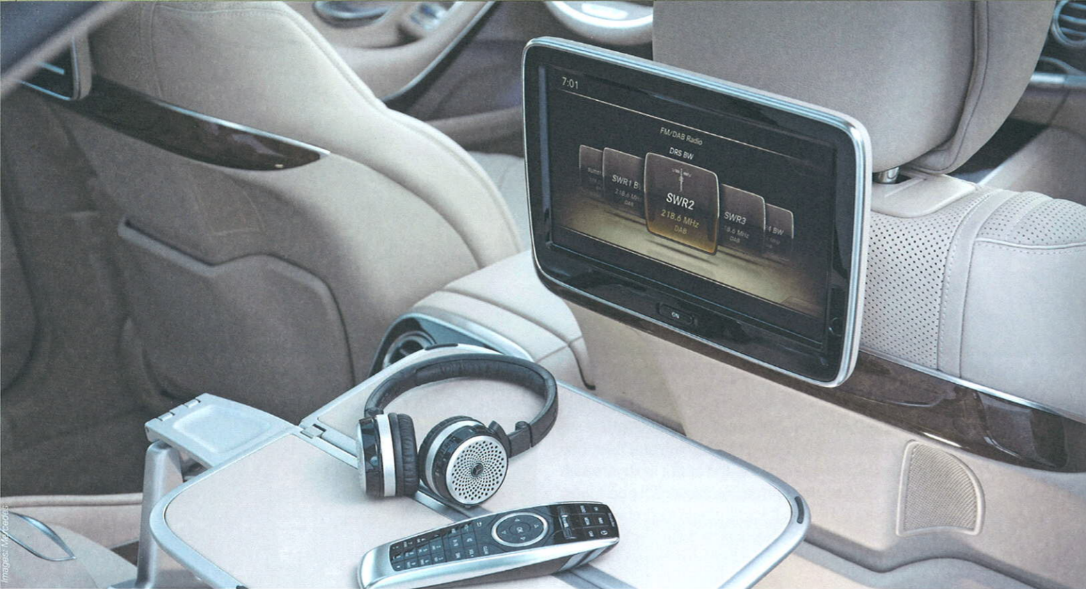
The colour displays are mounted on the headrests of the front seats for the rear-seat entertainment system.
