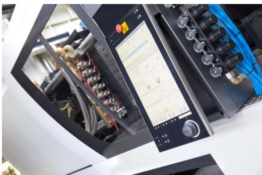
Integrated into the CC300 control of the e-motion injection molding machine, the iQ assistance systems compensate for process fluctuations in real time. (Image: ENGEL)
