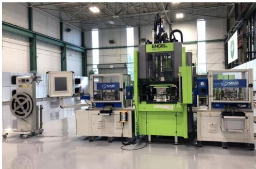
The highly-integrated process makes the production of thermal switch housings economically viable. Upstream of the injection process there are a strip uncoiler, a press module and a processing module for tapping a thread; downstream there are quality controls, laser marking and another press module. (Image: ENGEL)
