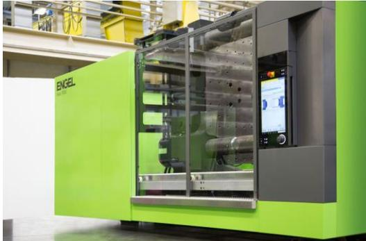
A duo 5160/1000 injection molding machine is being used for the production of ready to install door panels. (Image: ENGEL)
