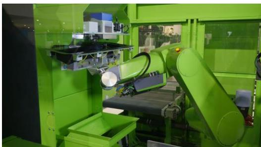
The easix articulated robot follows the component contour along the laser and finally places the ready to install door panel on the conveyor belt. (Image: ENGEL)
