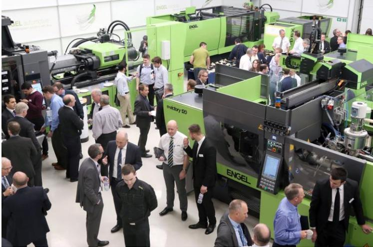
On the two days of the event, sample parts were injected using the MuCell process on an ENGEL e-victory 120. Vario-thermal mould temperature control ensured a premium, high-gloss finish.
