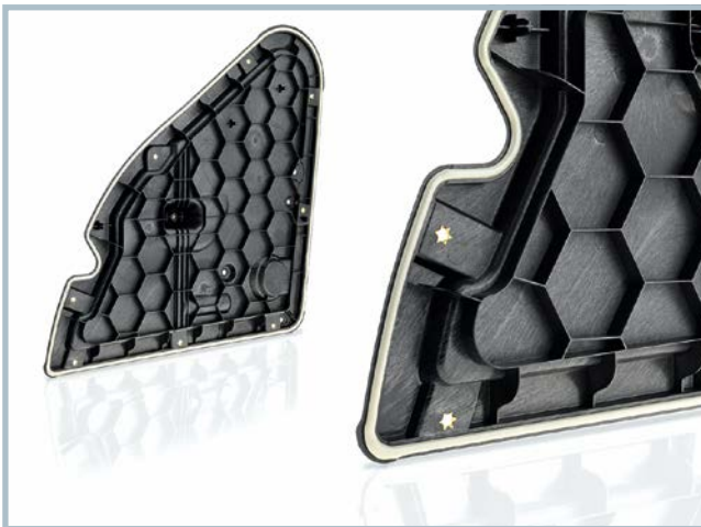
MuCell part with FIPFG gasket, metal rivets and thread insert: the door module for the Mini. Compared to non-foam injection molding, the required clamping force is a third lower (figures: KraussMaffei)
