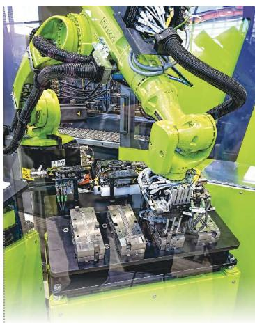
Engel showed automated changeover of mold inserts (front row on fixture) and robot EOAT (back row) in production of a two-piece caliper. In about 1 min, the robot changed EOAT from part handling to mold-insert handling (and vice versa), and then changed mold inserts to produce two different parts in alternating batches. The robot also placed matching pairs of parts into an assembly device and laser-marking fixture. (For more details, see October Keeping Up.)
