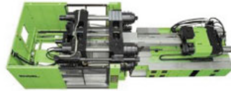
ENGEL offers the only two platen injection molding machine that has no contact with the tie bars, allowing frictionless movement to better control speed and precision
