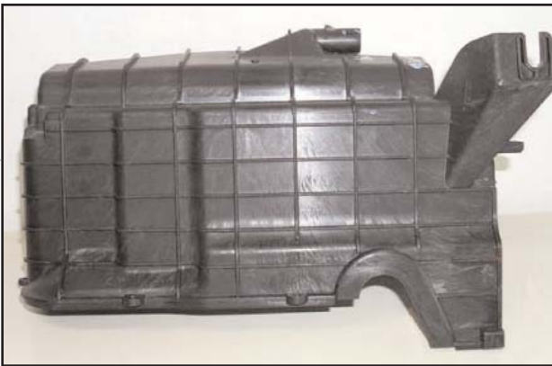
The Hyundai Avante/Elantra's HVAC housing utilizes the MuCell process to improve manufacturability, reduce noise and save weight.
