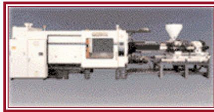
Milacron 400-ton Magna Hydraulic MuCell-equipped machine
