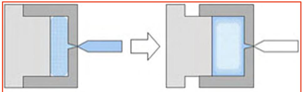
In core back molding, once the foamed resin has filled the mold, the volume of the mold is increased causing the foam to expand (see part cross-section).
